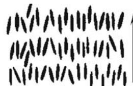
(a) Molecular arrangement in a SmA phase. The long axes of the molecules in each layer, on an average, are  $\perp$  to the layer containing the molecules.
