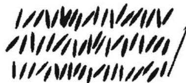
(b) Molecular arrangement in a SmC phase, the director makes an angle other than  $90^\circ$  with the layer planes
